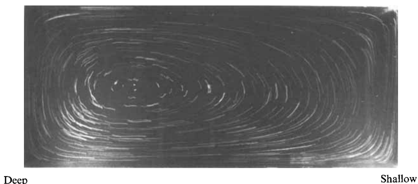
FIGURE 2. Streak photograph showing the starting flow of a homogeneous free-surface fluid in a rectangular tank with a sloping bottom that is spun-up from rest. Experimental parameters: \delta = 2.28 , \gamma = 0.34 , \alpha = 0.92 and the rotation period T = 11.3 s. The photograph was taken with exposure time 1 s.
